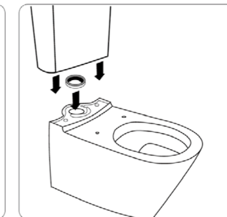
6 Install ceramic cistern.
